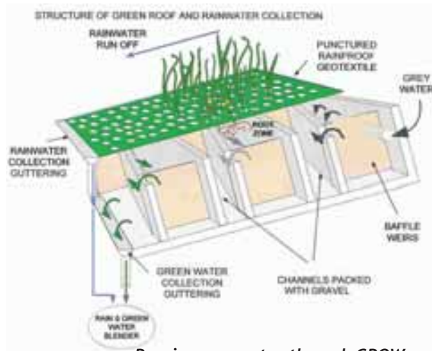
Reusing greywater through GROW system
